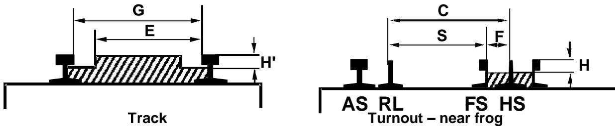
The horizontal dimensions of this standard are measured from the vertical edges of the rail profile.
